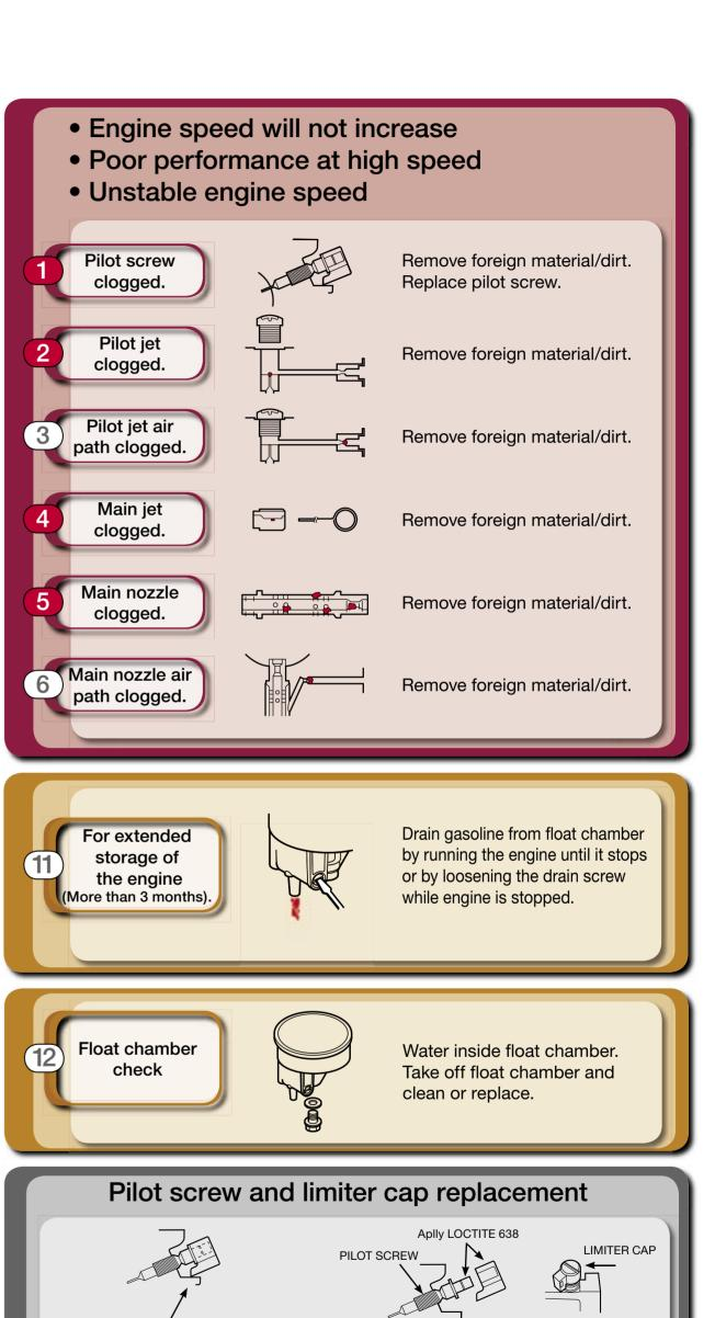
Install a new pilot screw and set it to
