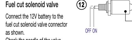
Check the needle of the valve should retract in.
